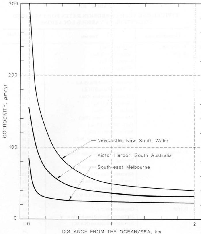
**GRAPHS DERIVED FROM MEASURED DATA SHOWING VARIATION OF ONE YEAR CORROSION RATE OF MILD STEEL WITH DISTANCE FROM THE OCEAN**
